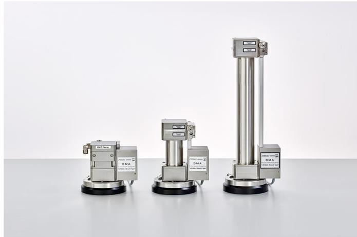
Figure 8. The GRIMM differential mobility analyzers.
