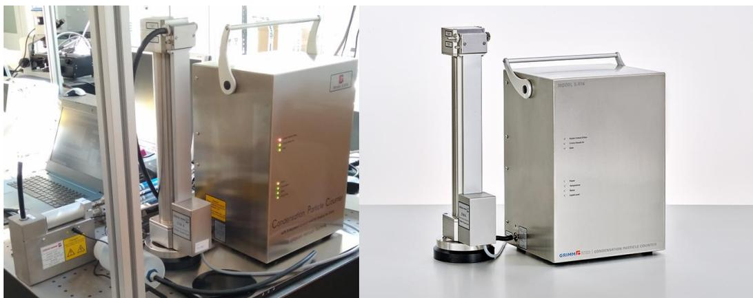
Figure 9. The GRIMM Scanning Mobility Particle Sizer (SMPS)
